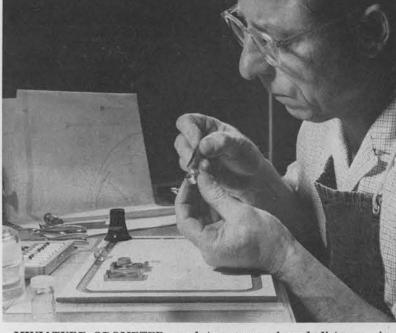
MINIATURE ODOMETER, used to measure lapsed distances, is being assembled by Ed Grymkowski. Large scale drawings, designed by engineering groups, have been used in tooling tiny parts.
